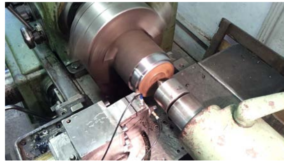
Fig.5. The stand to study the cutter vibration level using lathe tool holder with oriented center of rigidity when machining on the lathe 1K62
